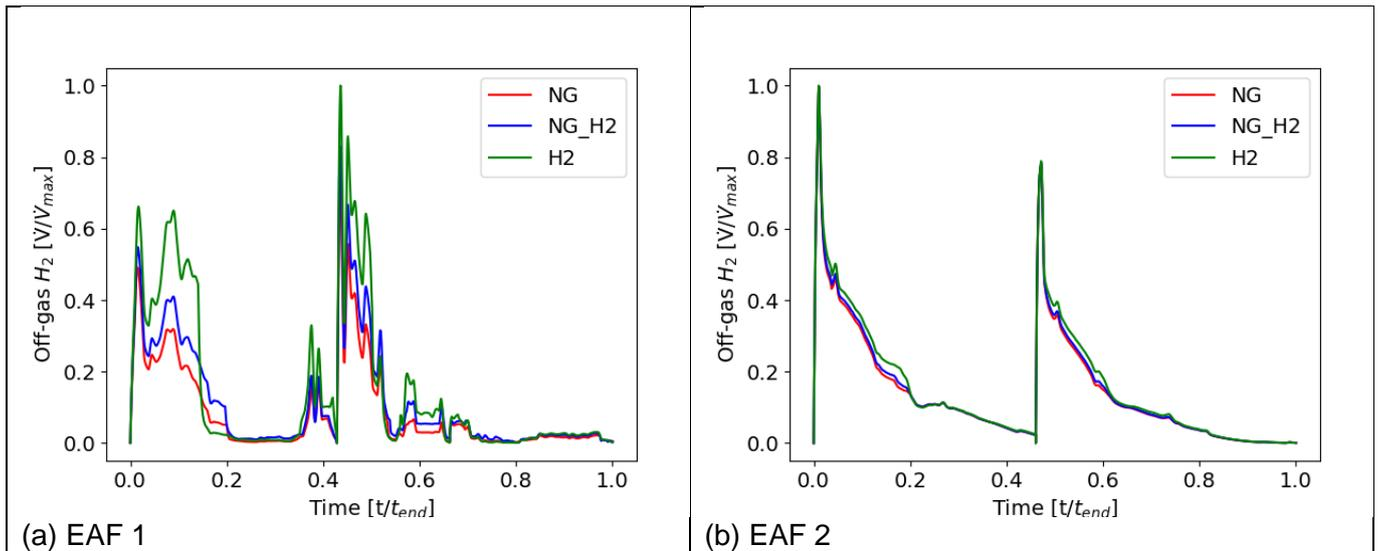
Fig 3: Hydrogen content of the off-gas during one heat
