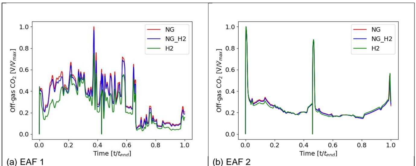
Fig 4: Carbon dioxide content of the off-gas during one heat
