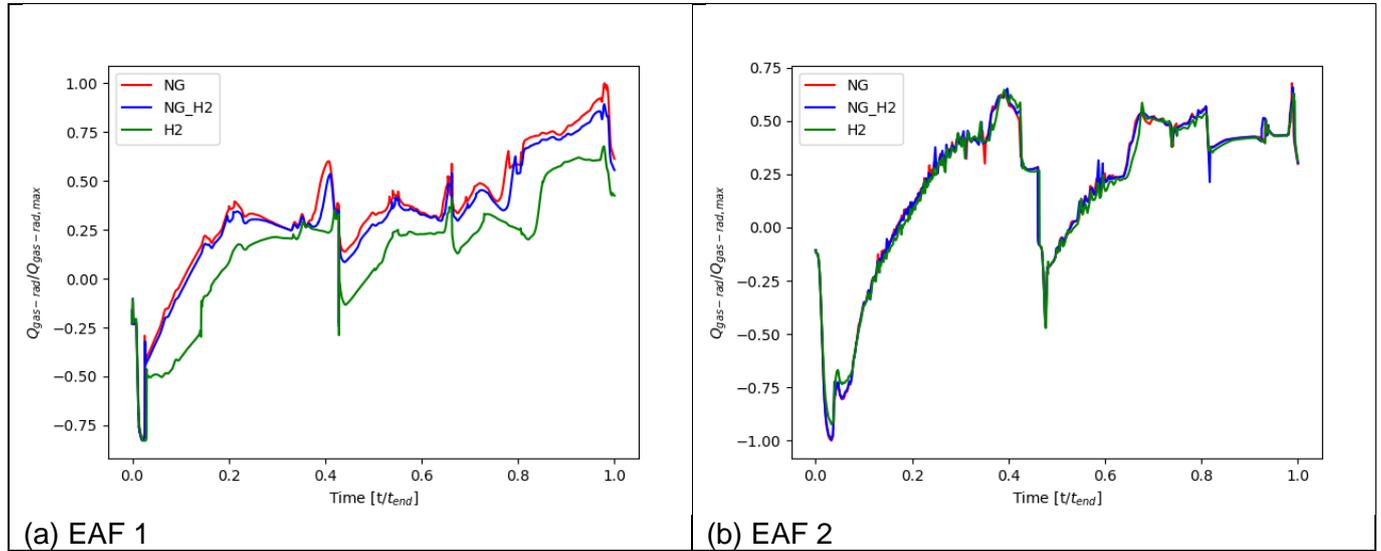
Fig 5: Radiative properties of the off-gas during one heat
