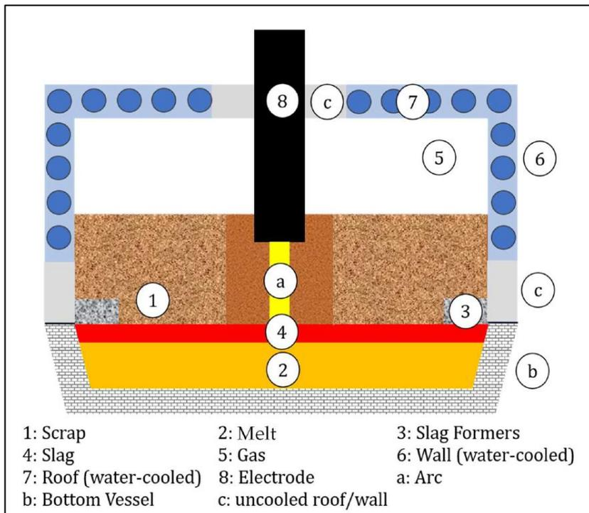
Fig. 1: Model zones (1-8) and heat sources/sinks (a-c) in the EAF process model <sup>[12]</sup>
