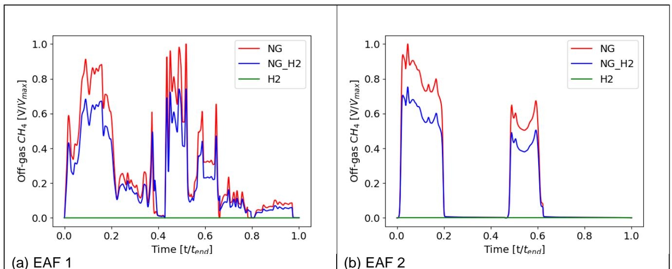
Fig 2: Methane content of the off-gas during one heat
