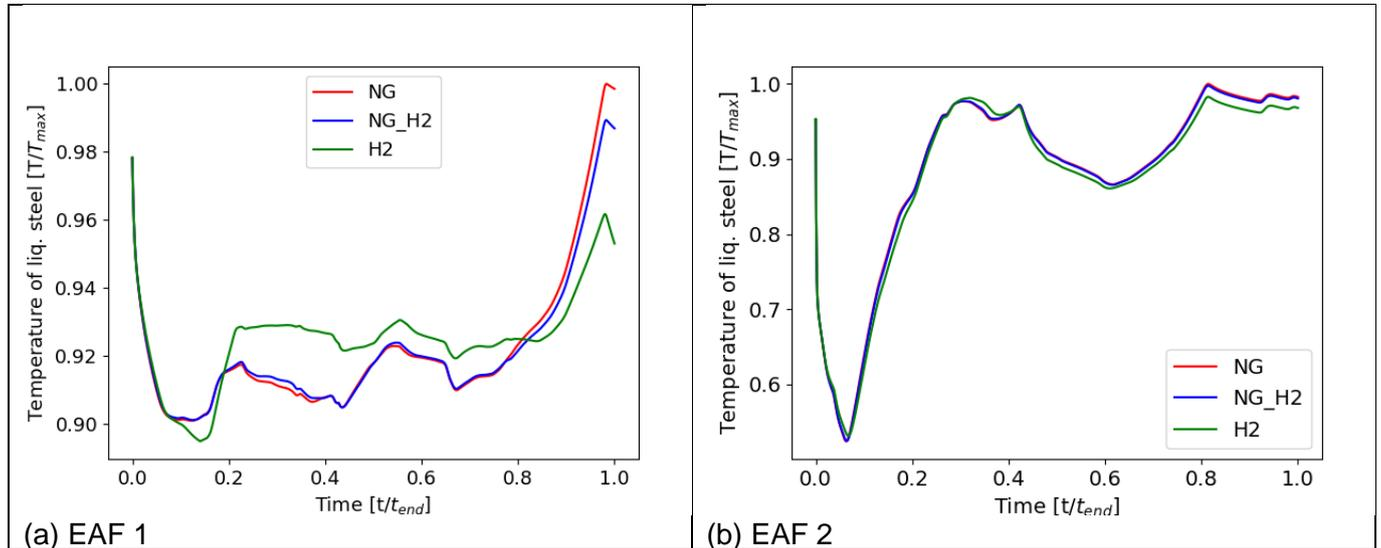
Fig 7: Temperature of liquid steel during one heat
