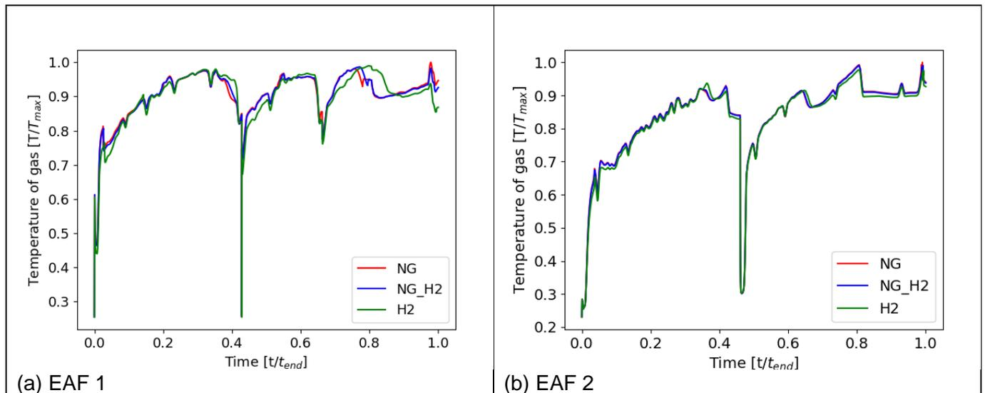
Fig 6: Temperature of the off-gas during one heat
